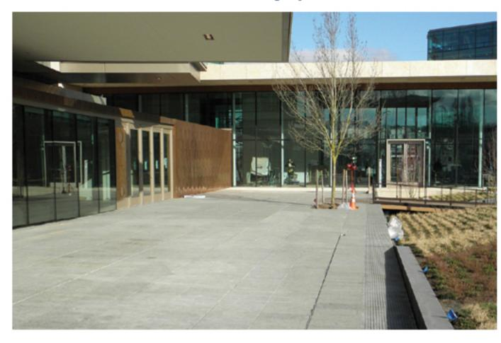
The Bill and Melinda Gates Foundation Campus features a 70,000-square-foot stone paver plaza, constructed with several Quikrete underlayment and grouting products. Quikrete Sand/Topping Mix was used for the two-inch-thick paver underlayment over a cast-in-place concrete slab for all exterior installations.
