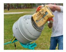
When **machine mixing**, concrete should be mixed in a barrel-type mixer. The mixing blades in a barreltype mixer are attached to the inside of the rotating barrel.
