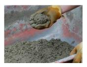
Properly mixed concrete should look like thick oatmeal and should hold its shape when it is squeezed in a gloved hand.
