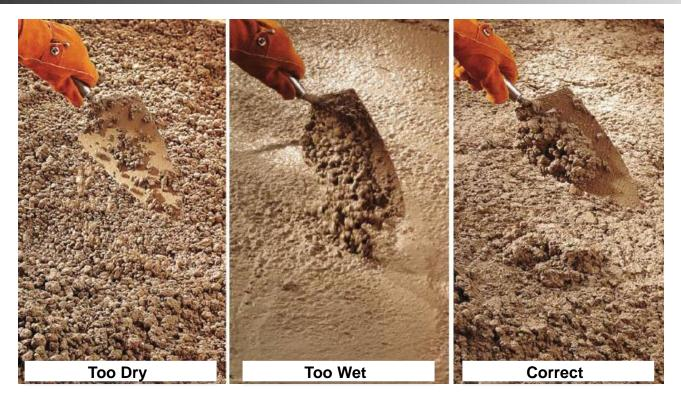
When mixing concrete, it is important to know that **the more water that is added to the mix**, **the weaker the concrete becomes.** Concrete is designed to reach specific minimum compressive strengths, based on the water addition instructions listed on the bag.
