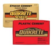
**Stucco Cement:** Blended cement for use with plaster sand (coarse stucco sand) to make base coat (scratch & brown coat) and finish coat (texture coat) stucco. **Plastic Cement** is a type of stucco cement used with plaster sand to make base coat stucco (scratch & brown coat).
