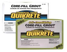
**Coarse Core-Fill Grout:** Use when grout space is greater than 4 inches in either direction. *Self-Consolidating Core-Fill Grout* is a type of coarse core-fill grout, and it meets ASTM C 476 at 24 – 48 (600 – 700 mm) in. slump flow. It contains coarse aggregate (3/8 in.).
