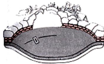
**7.** After the concrete loses its sheen, finish it with a trowel or wooden float.
