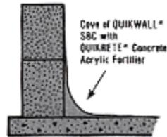
3. The remaining batches of QUIKRETE® Surface Bonding Cement do not require QUIKRETE® Concrete Acrylic Fortifier. Trowel the prepared QUIKWALL® on both sides and on the top of the blocks, taking care to completely cover them. One 50-pound bag is sufficient to cover an area of approximately 50 square feet to a depth of 1/8". The bed on top of the blocks should be a minimum of 1/4" thick.
