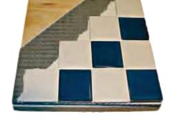
proof product comes in  $^{1}/_{4}$ - and  $^{1}/_{2}$ -inch thicknesses in 3x5, 4x4, and 4x8 sheets. Although ASTM testing isn't quite complete, it appears that the product performs better than conventional backers, especially at 19.2- and 24-inch joist spacing. The company says pricing runs about 45 cents per square foot.
