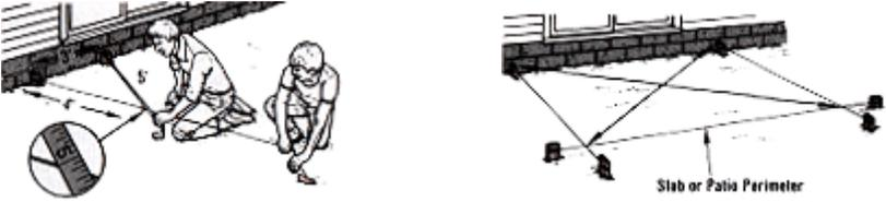
When deeper trenches must be dug for wall and foundation footers, it is best to lay out batter boards. Batter boards are set back from the actual work area so they are not disturbed by digging and construction. They also serve as a record of all important locations, such as trench and footer dimensions and the location of the outer edge of the finished wall. To lay out batter boards:
