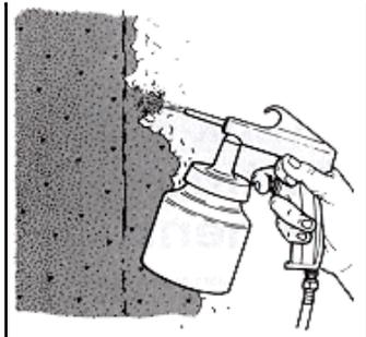
3. Apply the QUIKWALL® SBC in the same manner as described earlier. When relining silos, it is very important that the walls be troweled extra smooth to minimize the occurrence of small pockets where future acid crusting could originate.
